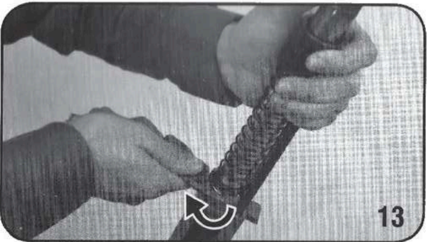
13. Remove the forearm connecting the barrel with the main body. (Turn Left side). The connector cap should always be checked before going to range and it shouldn't be loose.
